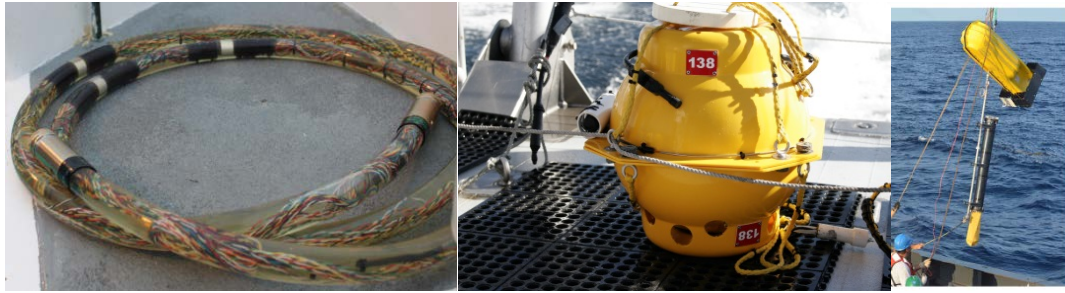
Figure 8-1 Examples of passive acoustic recording equipment employed during AMAPPS I Left side: active section of a custom-built towed hydrophone array. Center: Marine Autonomous Recording Unit (MARU, Cornell University). Right side: Autonomous Multichannel Acoustic Recorder (AMAR, Jasco Applied Sciences).
